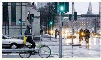
Figure 29. Junctions – resting rails provide support and convenience at junctions and have been implemented in Copenhagen, DK and are starting to appear in other cities such as Chicago, USA (Photo: Copenhagenize.com)
