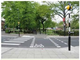
Figure 32. **Crossings** – parallel cycle and pedestrian crossing, Chapel Field North, Norwich. (Photo: Sustrans, UK).
