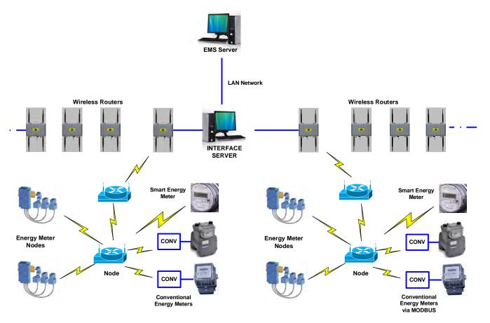
Multiple routers form a mesh network to connect various nodes (or areas) with the EMS server.
