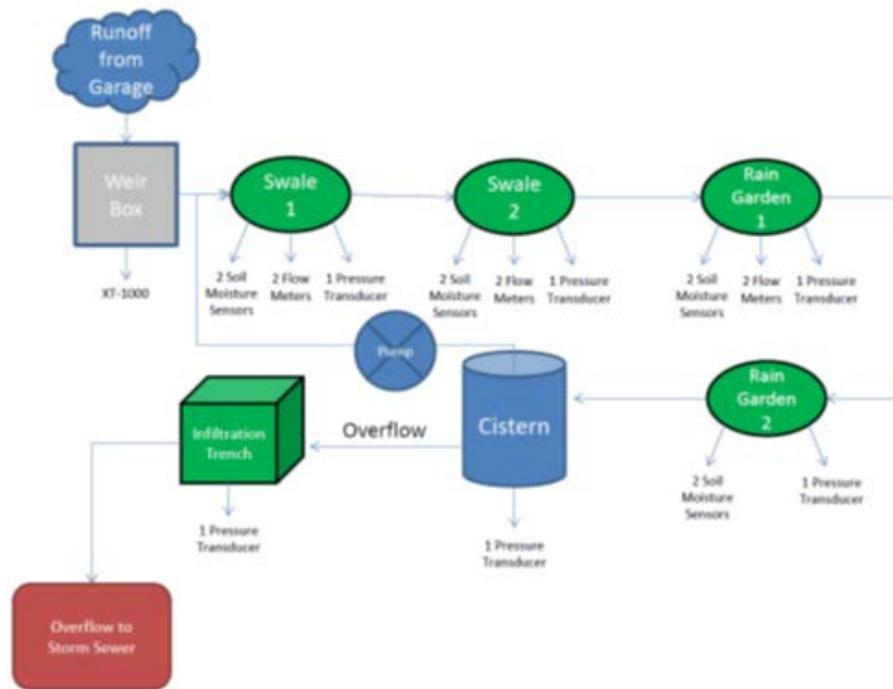
Figure 2: A schematic of the treatment train in 2016 with sensor locations.
