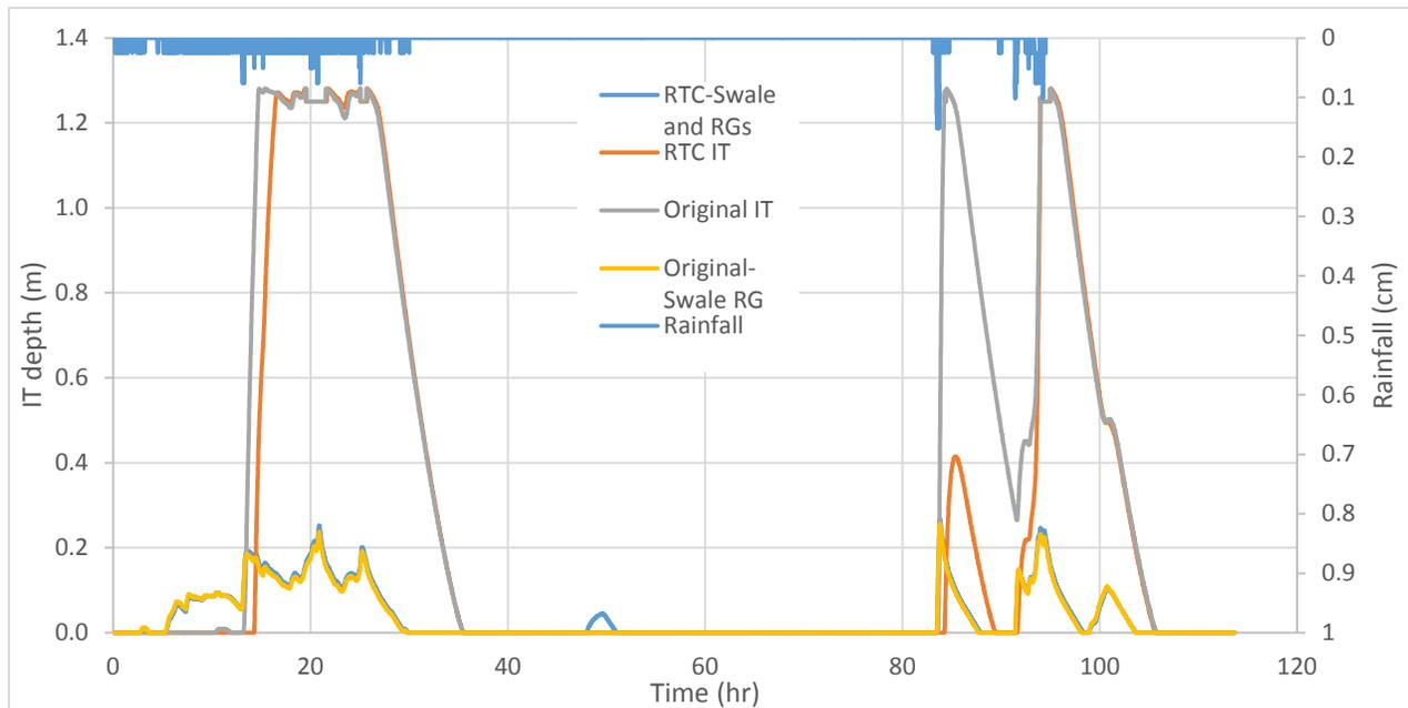
Figure 4: A comparison of passive and RTC treatment train performance for rain events occurring between June 6 (6:30 PM = time 0 hr) and June 10, 2013 (6:30 PM = 96 hr).
