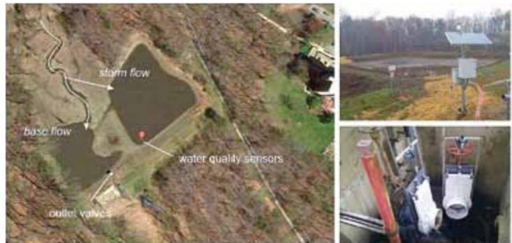
Figure 5. Aerial image of 15 acre-foot (18,500-cubic meter) retention pond with 440-acre (180-hectare) watershed on Sligo Creek in Montgomery County, Maryland (left); solar-powered control panel with cellular data connectivity (top right); and retrofitted outlet structure with actuated slide gate valves passing only baseflow (bottom right)
