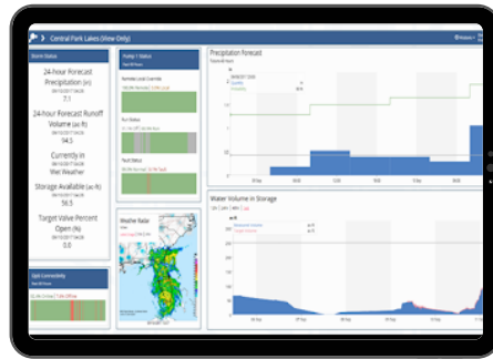
Comparison of forecast based management (blue) vs. traditional pump controls (red)
